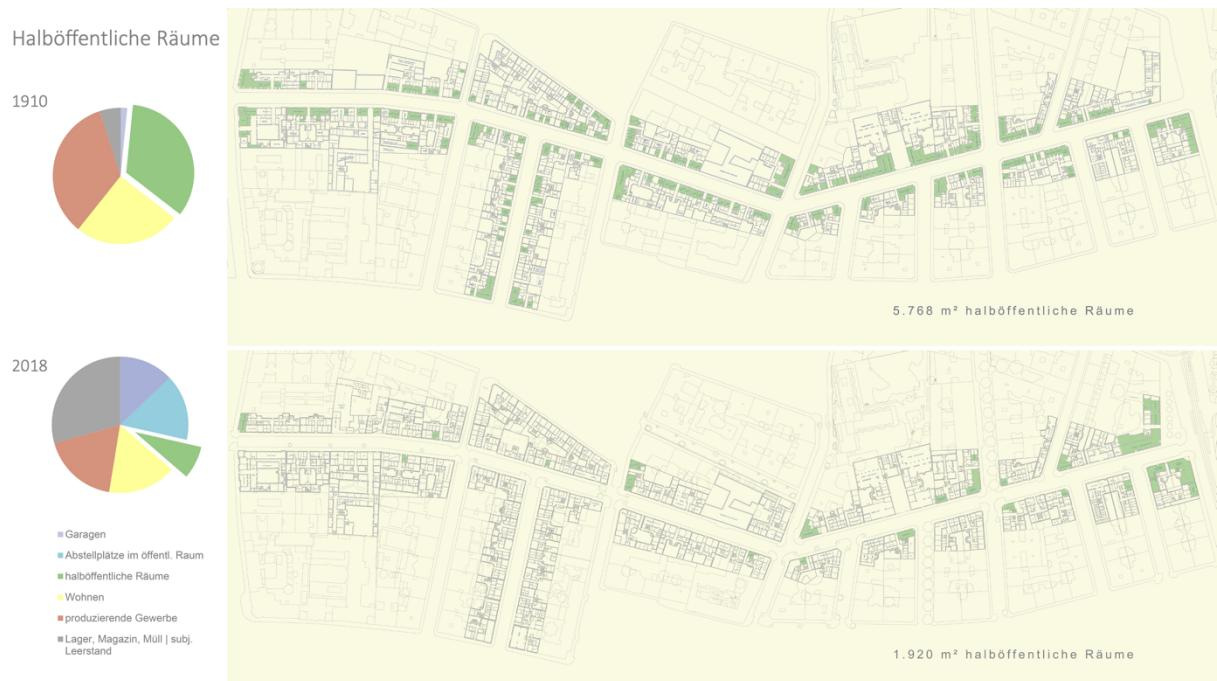
Fig. 4: The UPM allows a spatial usage structure analysis (Nutzungsstrukturanalyse) which—when the historical situation is compared with the current one—provides information on the different developments and interrelations. © Psenner 2019
